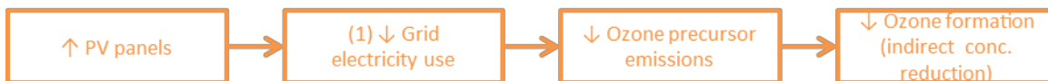
Figure 31. Rooftop PV ozone concentration reduction pathway (Note: Up arrows (↑) indicate an increase, and down arrows (↓) indicate a decrease)
